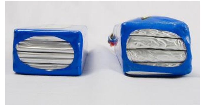
Battery swelling caused by overcharging
