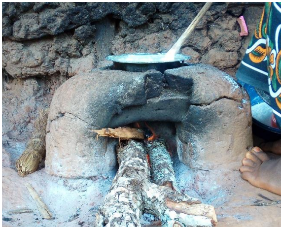
Figure 6. This a lorena stove (improved stove used by many households in Congo, Tanzania, Kalangala and kiboga
